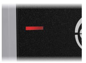
LED signaling on the inspection window: red indicates that a charging error has occurred.
