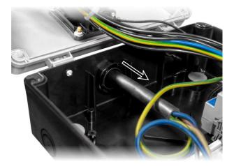
Insulate the end of the cable and crimp the individual conductors with sleeve lugs with a diameter that matches the conductor diameter. Connect all wires to the individual terminals located on the TH35 mounting rail:
