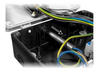
Insulate the end of the cable and crimp the individual conductors with sleeve lugs with a diameter that matches the conductor diameter.
