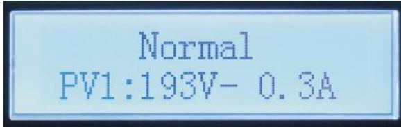
Inverter working status, PV generated power
