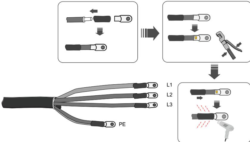
Step 5: Depending on the grid configuration, connect L1, L2, L3 and N to the terminals according to the label and tighten the screw on the terminal using a screwdriver.
