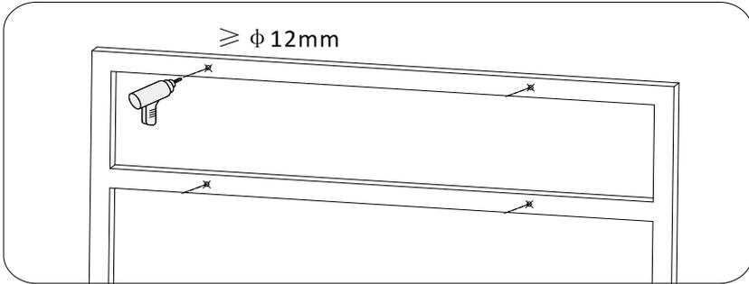
Figure 4-13 Drilling holes
