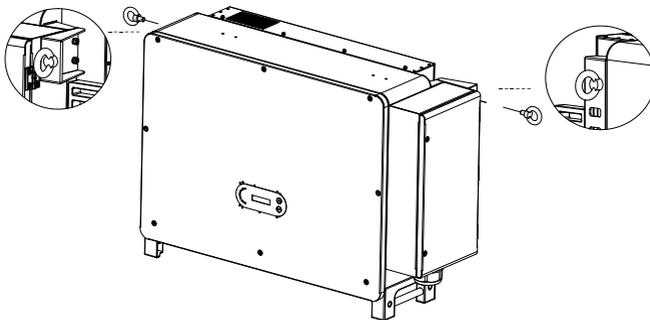
Figure 4-6 Installation of Rings
