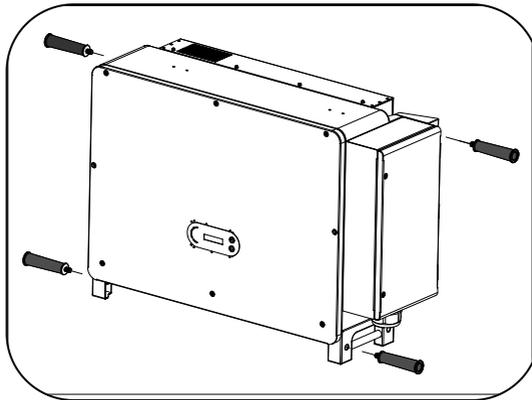
Figure 4-15 Installation position of auxiliary handle
