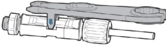
Figure 5-10 Removal DC connector
