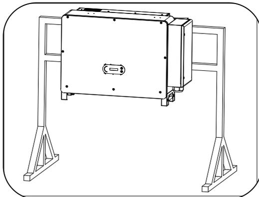
Note: If height between ground and bracket is less than 1.3m, use auxiliary handle for installation. Otherwise, use lifting equipment.
