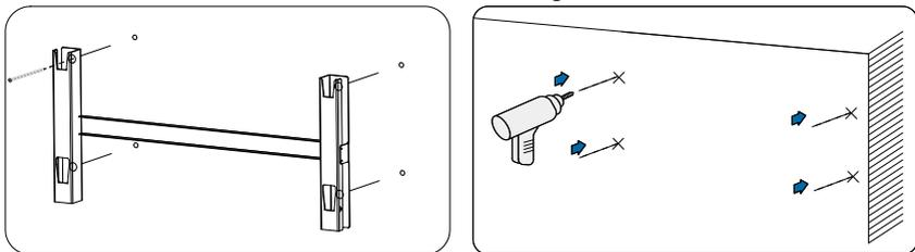
Figure 4-8 Drilling holes on the mounting wall
