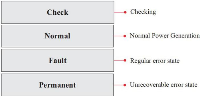
Inverter states includes: wait, check, normal, fault and permanent.
