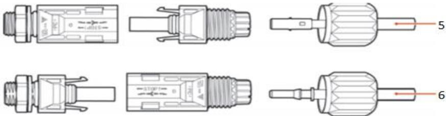
Figure 5-9 DC cable connection
