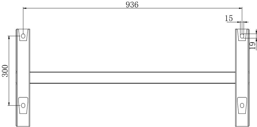
Figure 2-3 Product back view and bracket dimensions
