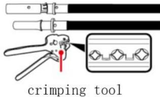
Step 3: Insert wire into the connector cap nut and assemble into the back of male or female plug, When you heard a “click”, the pin tact assembly is seated correctly. (3. Positive Connector, 4. negative connector).
