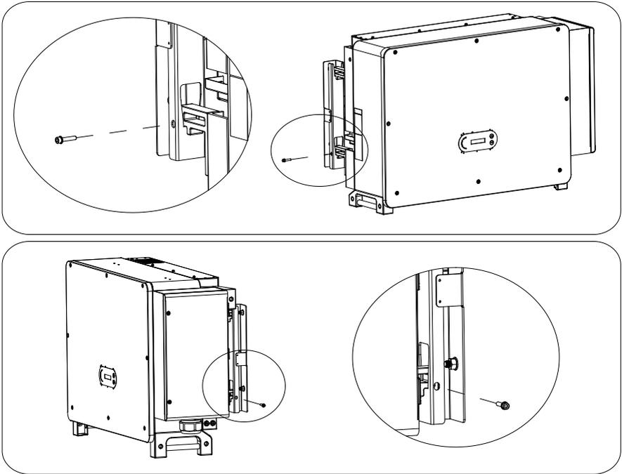
Figure 4-11 Fix inverter
