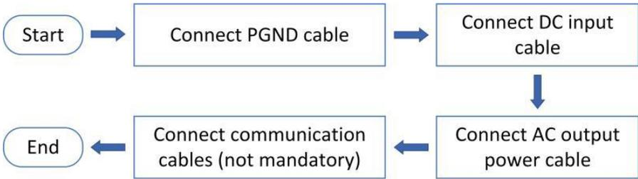
Figure 5-1 Flowchart for connecting cables to the inverter
