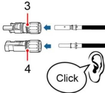
Step 4: Measure PV voltage of DC input with multimeter, verify DC input cable polar and connect DC connector with inverter until hearing a slight sound indicated connection succeed.
