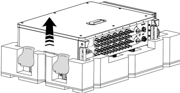
Figure 4-4 Move inverter from package
