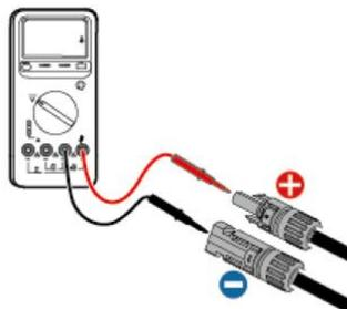
**Note :** Please use multimeter to make sure the PV array positive pole and negative pole!
