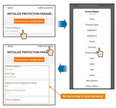
Figure 7-4 Initialization protection parameter
