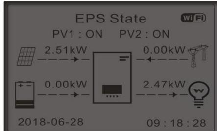
3) If PV generation < LOAD consumption ( $\Delta P > 100W$ ), inverter will discharge battery.
