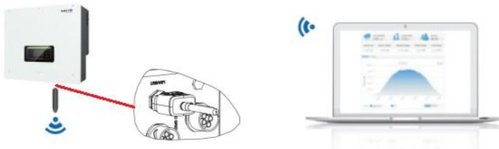
The operation information (generated energy, alert, operation status) of the inverter can be transferred to PC or uploaded to the server via WiFi/GPRS. Users can choose to use web or APP for monitoring and viewing according to their needs. They need to register an account and bind the device with the WiFi/GPRS SN number. The SN number of the WiFi/GPRS shall be affixed to the package box and the WiFi/GPRS.
