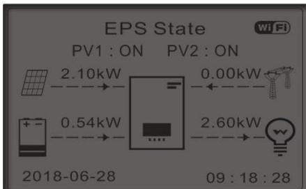
4) If PV generation is normal, but LOAD consumption=0, the surplus power will be stored in the battery.
